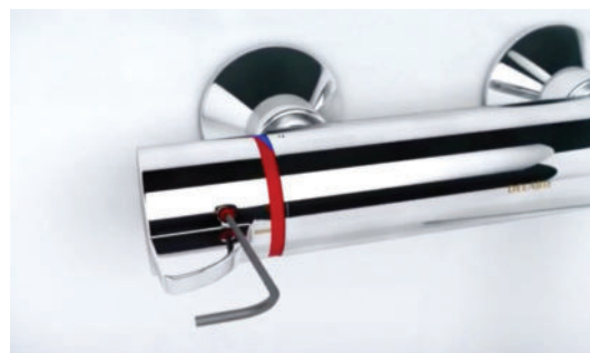
Unblock the maximum temperature limiter to carry out a thermal shock: simply push in the red button with a pointed tool.
