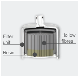
Section of the BIOFIL tap filter
